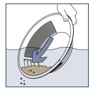
Repeat steps 3 to 5, progressing through the panning zones until the material has reduced significantly, leaving behind a concentrate of fine silt, tiny pebbles, black sand and gold.
